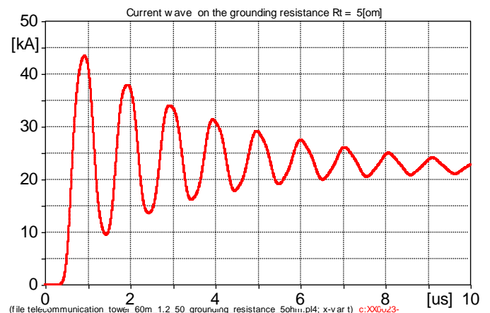
Fig. 9 Current waves on grounding resistance with R_t = 5 [ \Omega ] for standard wave 1.2/50 [ \mu s] lightning current sources, with peak current 100 [kA] on top of the tower
