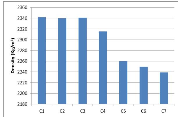
Fig. 7. Density test results of concrete mixes at age of 28 days.
