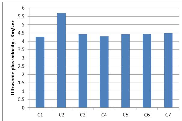
Fig. 6. Ultrasonic pulse velocity test results of concrete mixes at age of 28 days.
