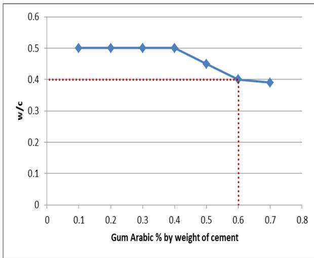
Fig. 1. w/c of concrete mixes which contain Gum Arabic
