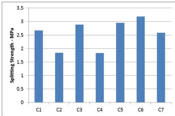
Fig. 4. Splitting strength of concrete mixes at age of 28 days .
