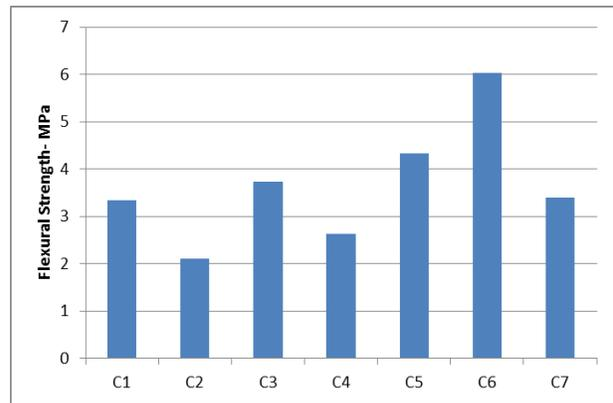
Fig. 3. Flexural strength of concrete mixes at age of 28 days .
