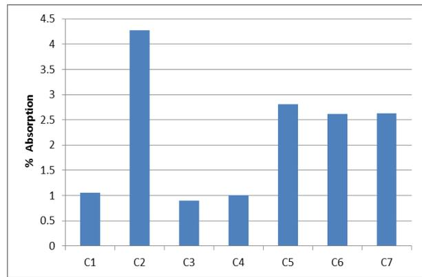
Fig. 5. Absorption test results of concrete mixes at age of 28 days.
