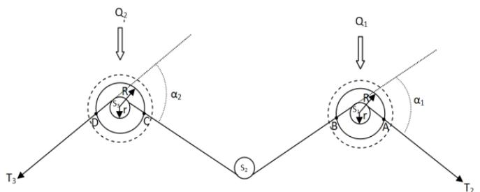
Fig. 4. Detailed tension variation across two disc tension devices and fixed post thread guide
