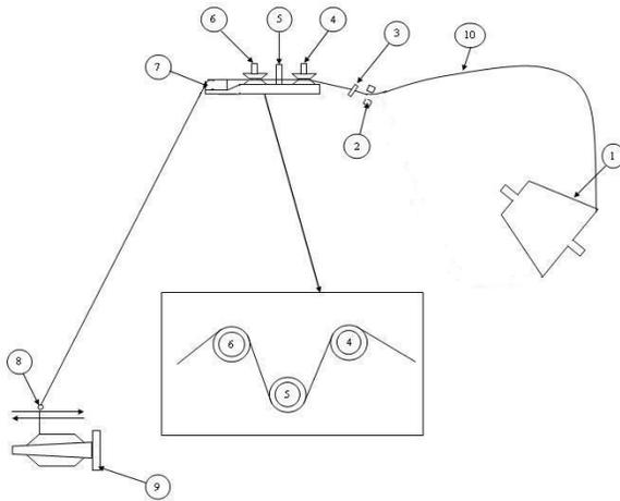
Fig. 2. Yarn path of pirn winding machine
