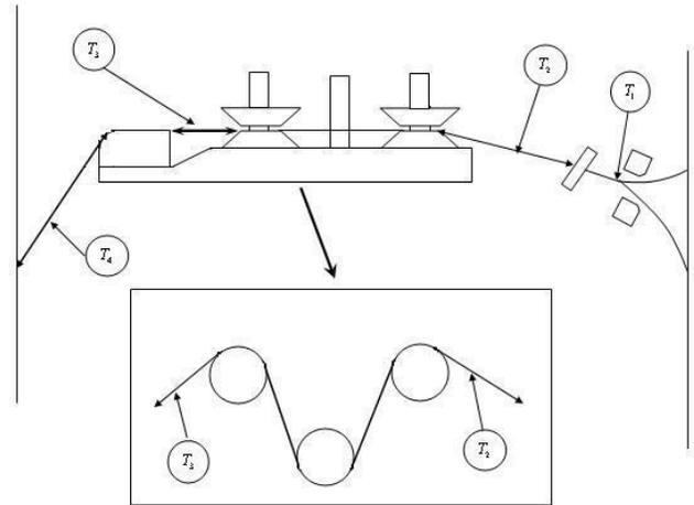
Fig. 3. Tension in different areas of the yarn path
