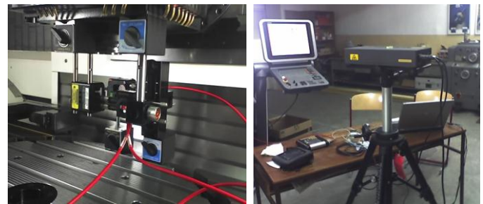
Fig. 7. Real time setup for straightness measurement (left – optics, right – laser head)
