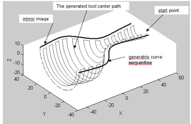
Fig. 10 The simulated tool center path for an axisymmetric die cavity with a serpentine as generatrix curve.
