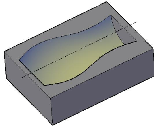
Fig. 1. Definition of an axisymmetric die cavity
