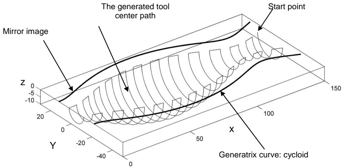
Fig. 7. The simulated tool center path for an axisymmetric die cavity with a cycloid as generatrix curve.
