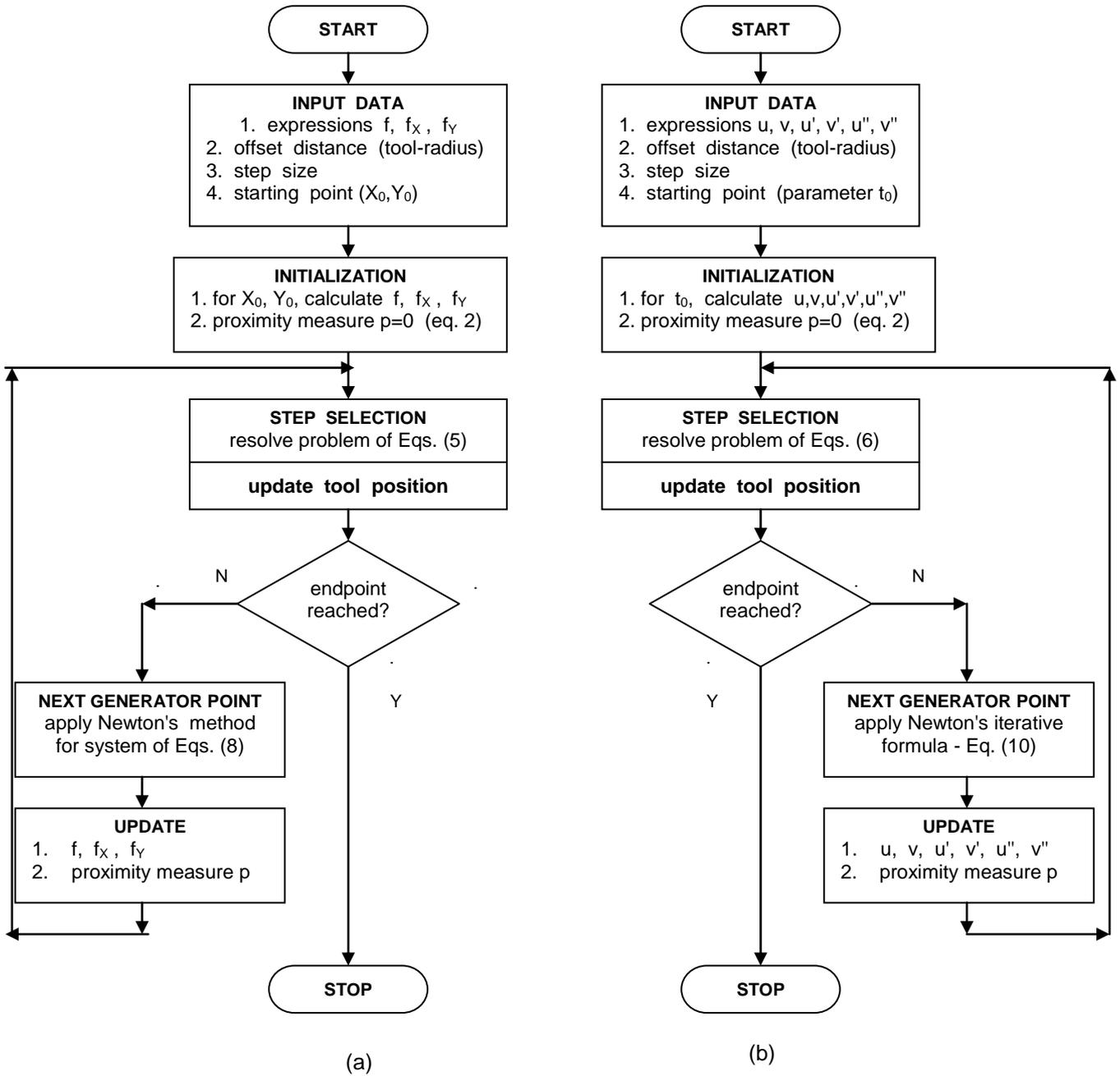
Fig. 4. Flow charts of the offset interpolator program. (a) for implicitly defined generators. (b) for parametrically defined generators
