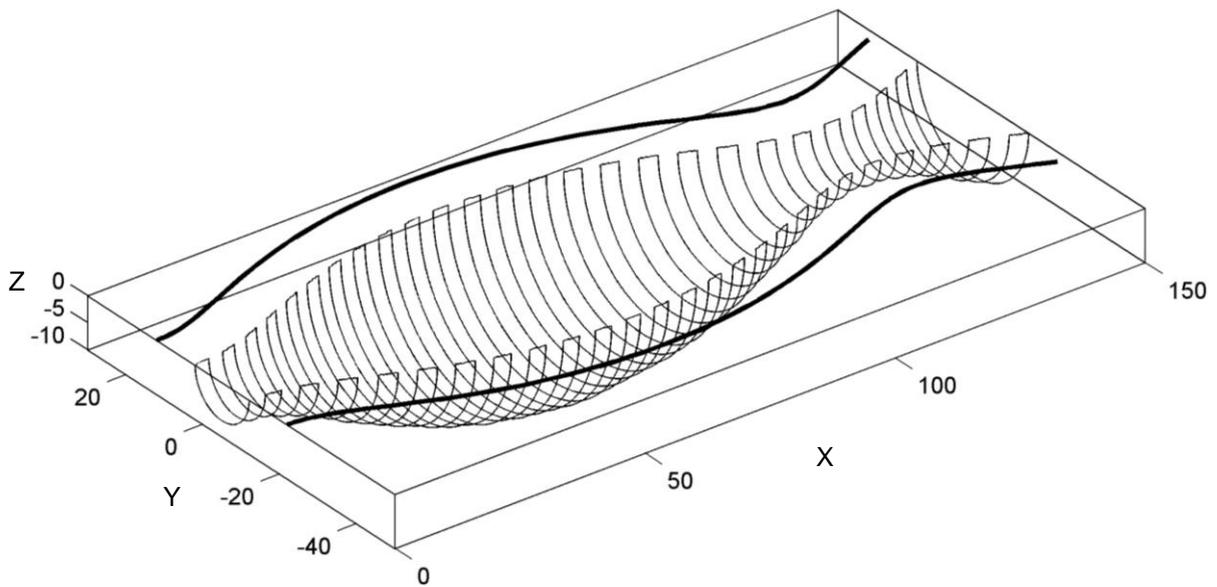
Fig. 8: The same die cavity as in Fig.7 with smaller distance between scallops
