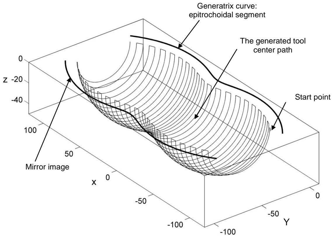
Fig. 11. The simulated tool center path for an axisymmetric die cavity with an epitrochoidal segment as generatrix curve.
