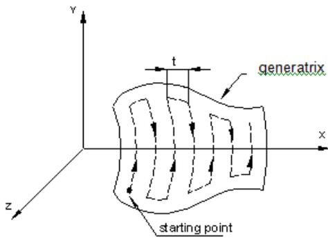
Fig.5. Tool center path for a revolved surface
