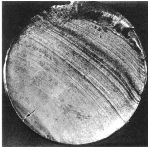
Figure.1. Fatigue crack surface. [2]
