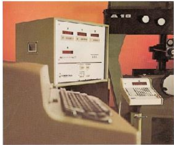
Fig.3: Wild EK22 Connected to a Wild A-10 Universal Stereoplotter.
