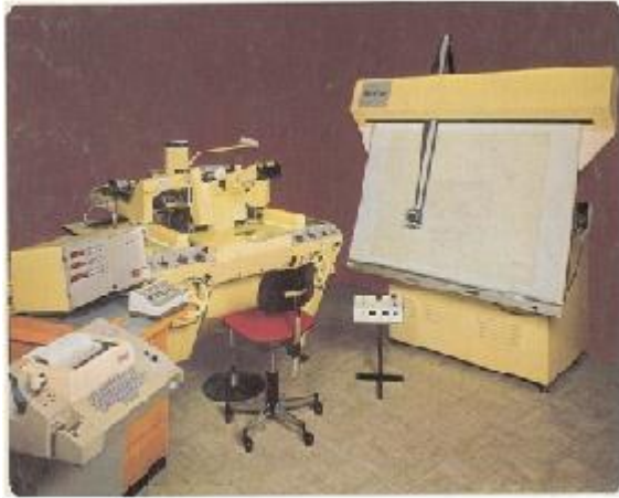
Fig.2: Data Acquisition System ER2 connected to a Kern PG-2 Topographic Stereoplotter.
