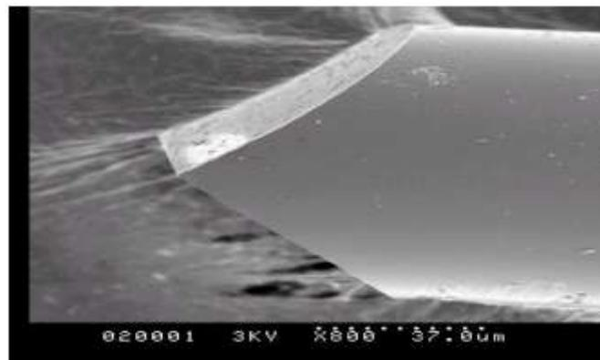
**Fig. 11. SEM photograph of wedge fiber endface**
