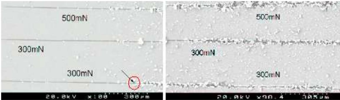
Fig. 1. Nano scratches on optical fiber material
