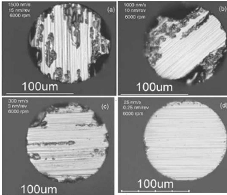
**Fig. 7. Optical fiber endfaces ground with 3  $\mu\text{m}$  grits**
