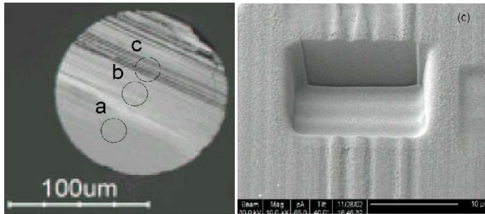
**Fig. 8. SEM photograph for a hole drilled using FIB on a ground optical fiber endface (region C)**
