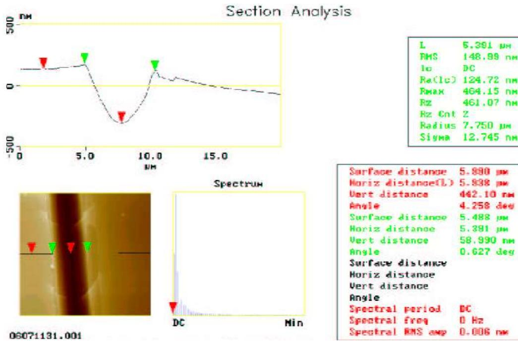
Fig. 2. AFM section analysis showing critical depth of cut if 442 nm.
