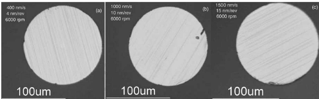
**Fig. 5. the effect of infeed rate on surface quality**
