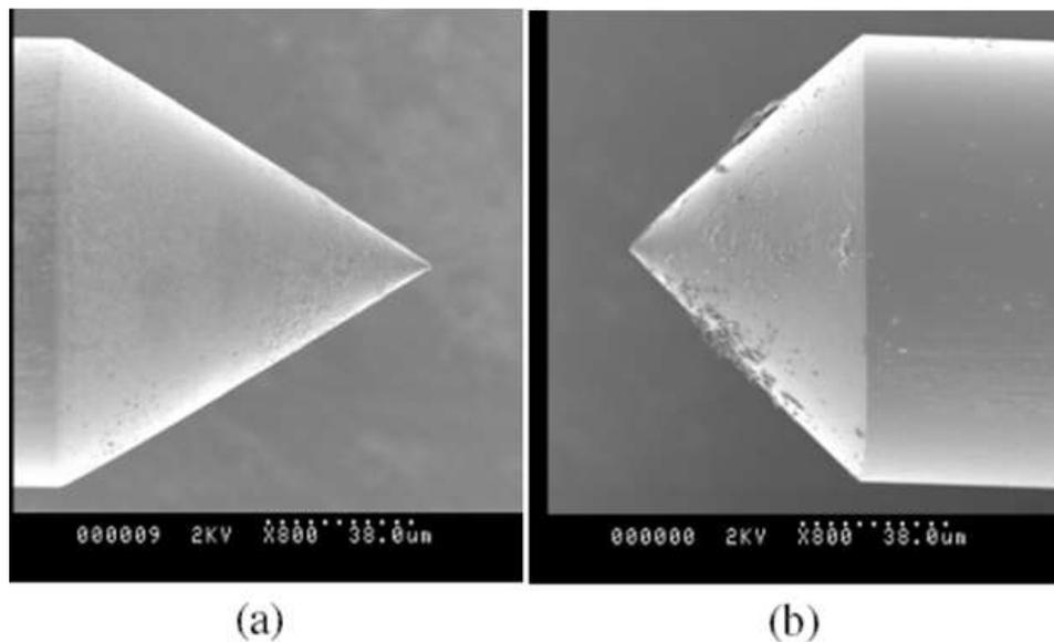
**Fig. 9. SEM photographs for ground conical lenses made using NGM: a) cone angle  $68^\circ$ , b) cone angle  $90^\circ$**
