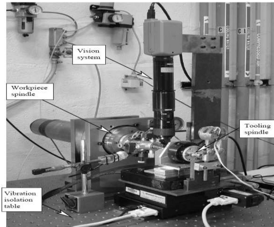
**Fig. 3. Photograph of the nano-grinding machine (NGM)**
