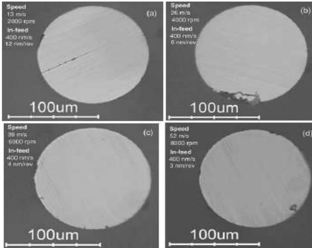
**Fig. 4. The effect of spindle speed on surface quality**
