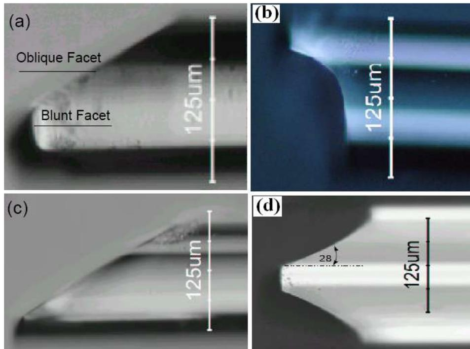
**Fig 10. Different optical fiber endfaces profile made using NGM a) oblique profile, b) D-shaped profile, c) slant profile, and d) wedged profile.**
