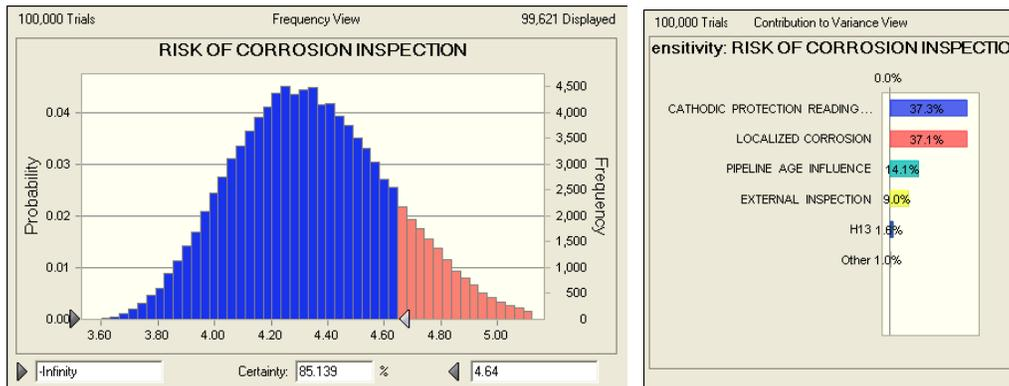
Figure 4: Forecast Corrosion Inspection and Sensitivity
