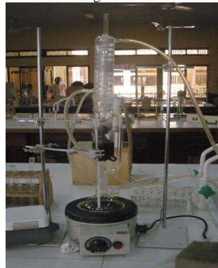
FIG. 1: Experimental Setup of Extraction Apparatus
