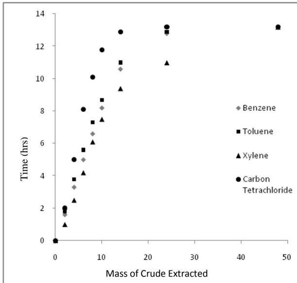
Fig. 2: The Graph of Time of Extraction and Mass of Crude Extracted.
